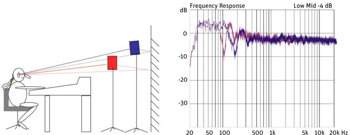
Increasing the distance of the loudspeaker from the wall increases the affected wavelength and therefore decreases the affected frequency (red example above). The loudspeaker should be positioned sufficiently far from the wall to locate this frequency below the loudspeaker/subwoofer crossover, so that any cancellation will be compensated for by the subwoofer.
