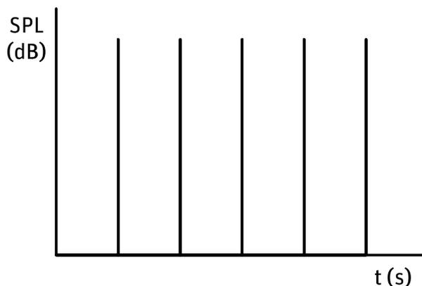
In some situations it is possible for the main loudspeaker and subwoofer to be in-phase at the crossover frequency, but have a delay between them of one or more cycles at the listening position. This causes impulsive sounds to be smeared in the time domain. The following plots show a low-pass filtered Dirac impulse with and without a one cycle delay at 80 Hz (12.5 ms) between the loudspeaker and subwoofer at the listening position.
