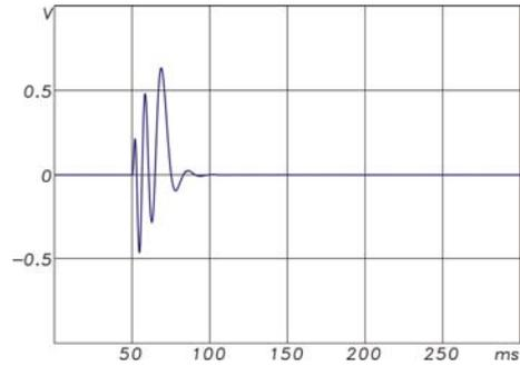
**Impulse response with 12.5ms (80 Hz) delay
